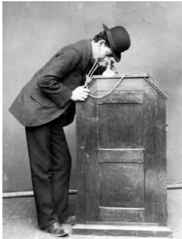
0-7 Kinetoscope with Phonograph cylinder audio player built in and earphones, 1895. Photo from victorian cinema.net
